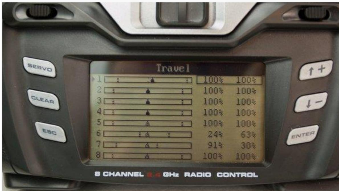
THIS MENU FOR EPA (CALLED "TRAVEL" BY TACTIC) SHOWS WHERE I HAD TO LIMIT THE SERVO MOVEMENT TO MAKE THE FLAPS AND BOMB RELEASE (CHANNELS 6 AND 7) FUNCTION PROPERLY ON THIS MODEL.
