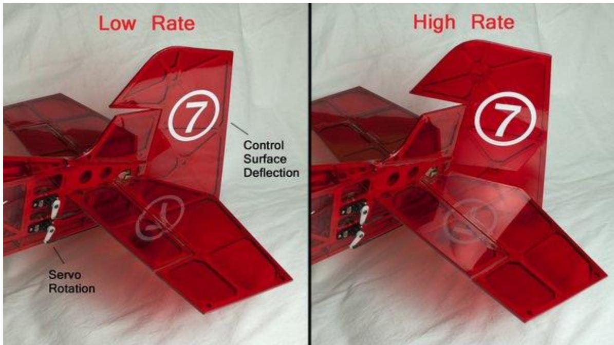
THIS MODEL HAS SIGNIFICANTLY GREATER RUDDER THROW (AND EXPO) IN HIGH RATE THAN IN LOW RATE. IT IS EASY TO SEE HOW THE INCREASED CONTROL SURFACE MOVEMENT WILL AFFECT THE AIRPLANE'S MANEUVERABILITY.
