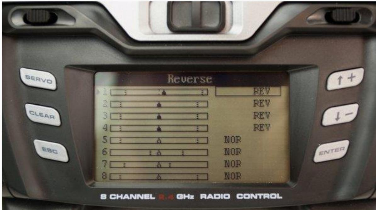
SERVO REVERSING IS A SIMPLE BUT VITAL FUNCTION FOR CONFIGURING THE CONTROL SYSTEM OF ANY MODEL. IMPROPER CONTROL MOVEMENT CAUSES MANY CRASHES.
