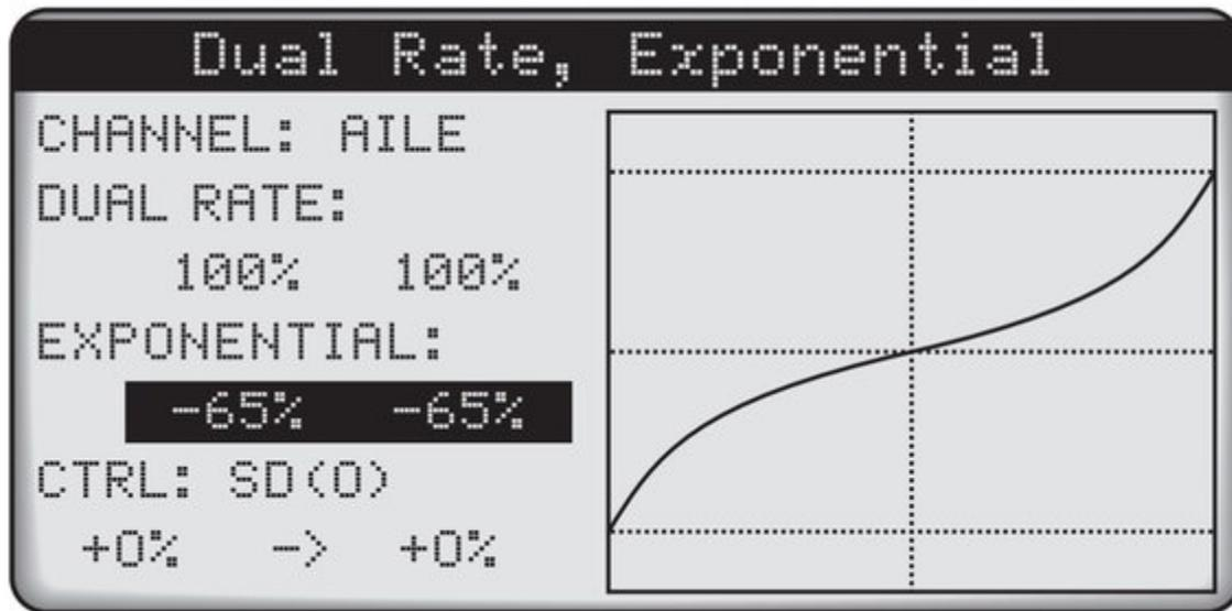
THIS DIAGRAM TAKEN FROM THE MANUAL FOR THE TACTIC TTX-850 RADIO ILLUSTRATES THE EFFECT OF EXPONENTIAL SETTINGS. THE X-AXIS IS CONTROL STICK MOVEMENT AND THE Y-AXIS IS SERVO MOVEMENT.
