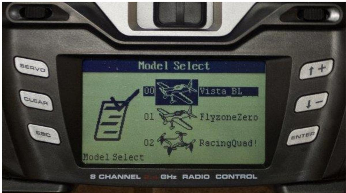
BIG APPEAL OF COMPUTER RADIOS IS THEIR ABILITY TO OPERATE MULTIPLE MODELS. YOU DON'T NEED A SEPARATE TRANSMITTER FOR EACH AIRCRAFT.
