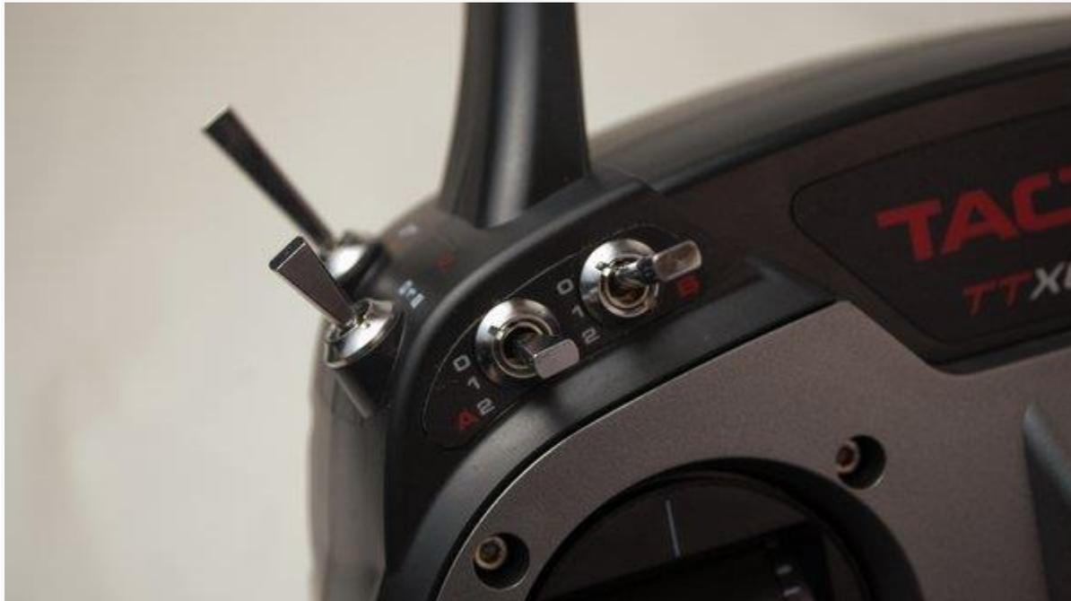
THE SWITCHES ON A TRANSMITTER CAN BE ASSIGNED TO CONTROL DUAL RATES. THIS LETS YOU ALTER THE SENSITIVITY OF YOUR MODEL WHILE IT IS FLYING.
